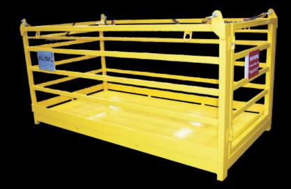
This unit is sized to accommodate a stretcher bound person and 2 attendants. The unit carries forged Harris Walton fixtures for attachment of a safety harness and fully internal handrailing. Supplied with 5.5mtr dedicated multileg chain sling to suit. Gate opens outward to facilitate stretcher loading.
